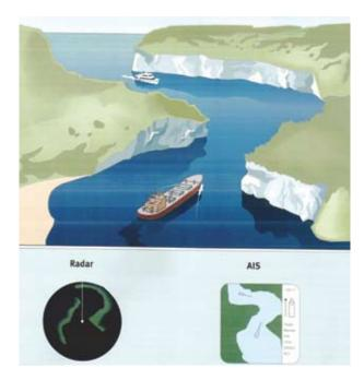
AIS is a system that provides data from all ships or devices fitted with an AIS Transponder. Received AIS data can be presented on electronic charting software and many of today's radars can overlay AIS data on the radar display to uniquely identify a radar target. AIS display over radar is the most effective way to present AIS targets and will become the most common application of this technology.
