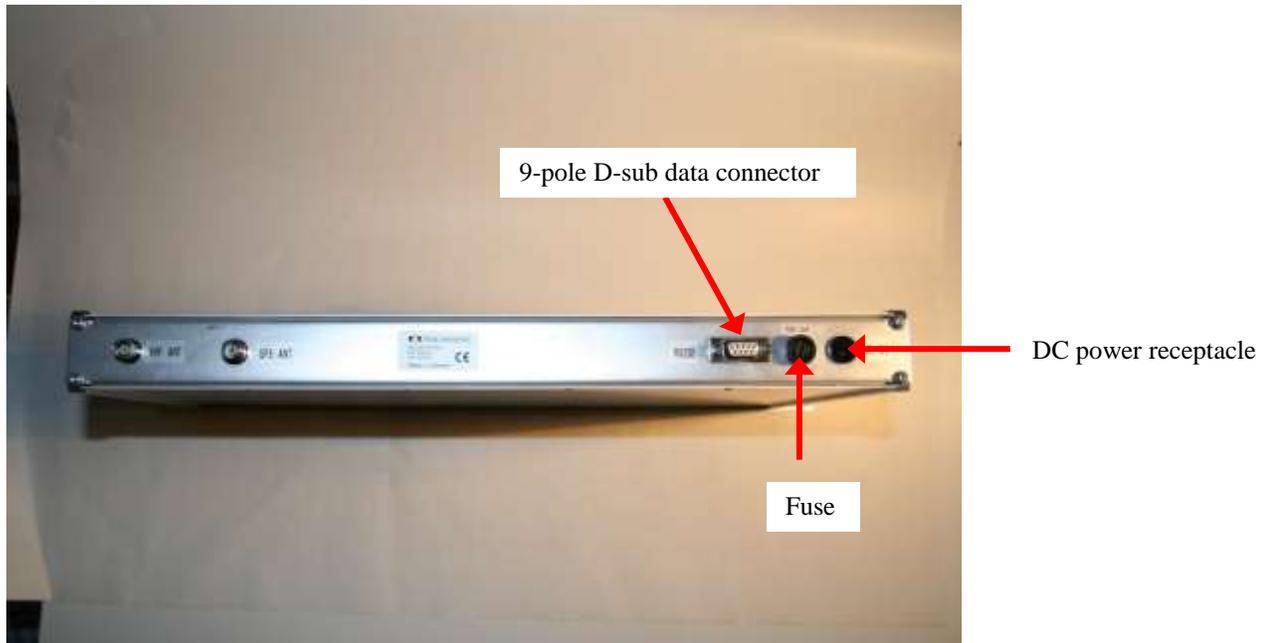
Figure 5 19" rack version, rear panel connections
