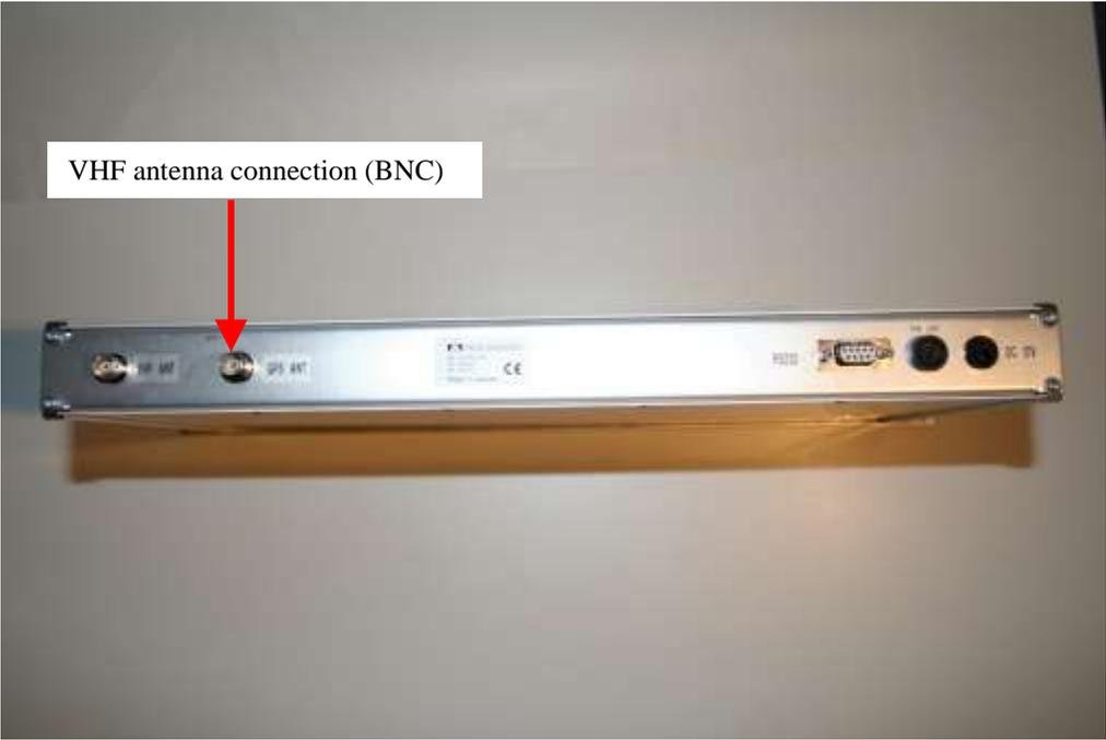
Figure 3. VHF antenna connection, 19" rack version.
