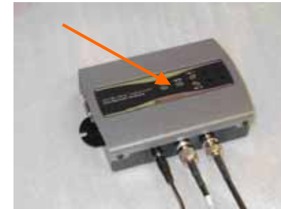
Picture 2 Power and antenna connections.
