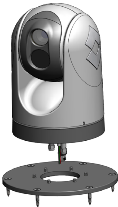
Top down installation using mounting plate
