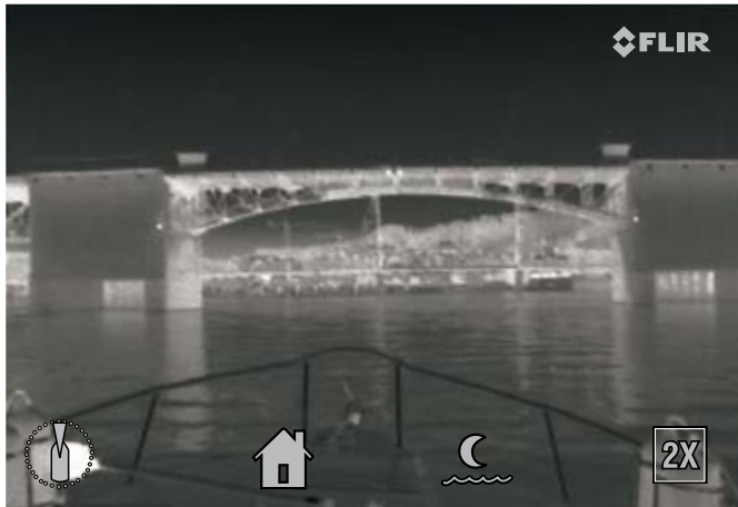
Thanks to small icons conveniently placed at the bottom of the thermal image, the captain can see immediately in which direction the Navigator II is looking, whether it is in the "home position" or not. Also other settings of the camera can easily be read from these icons.
